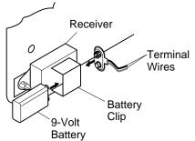
Figure 30 - Installing Receiver on the Back of the Base Continued
